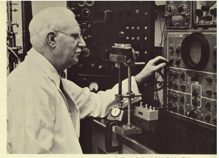
Dr. Alexander Sandow, chief of the Physiology Division, at the dual beam cathode-ray oscillograph, an apparatus which can measure muscle responses lasting only a fraction of a thousandth of a second.
