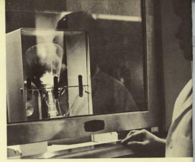
A sample of human tissue, containing a fraction of a part per million of selenium, is reduced to ash in an oxygen-filled combustion flask.
