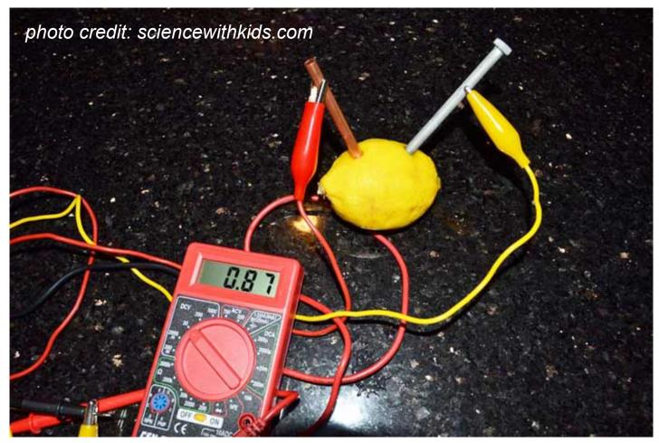
A galvanized (zinc-coated) nail and a copper tube are shown here inserted (not touching) into a lemon, and connected via alligator clips through a multimeter reading 0.87 V. Identify the key components of this electrochemical cell by name.
