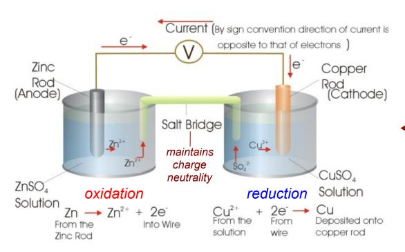
That's a short circuit. If you don't let the solution contact the copper directly, you can still flow electrons from zincto copper, using the spontaneity of the reaction to do work (remember free energy defines the maximum extractable non-PV work?)
