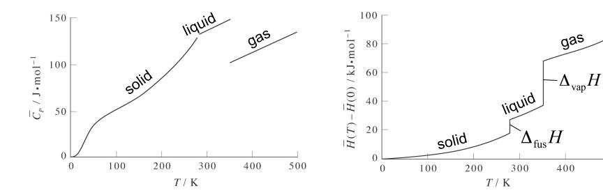
Measuring the heat capacity, temperature by temperature
