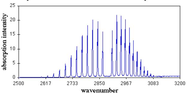
Quantum mechanics tells us that vibrational energy levels are quantized, and that the energy separations between levels are dictated by the shape of the potential within which vibration takes place (i.e., the 1-D PES). By observing the allowed (above, with rotational information too) and forbidden (not shown) transitions of HCl and its isotopomers (which have different vibrational energy levels by virtue of having different reduced masses) the shape of the PES can be deduced over a large range.
