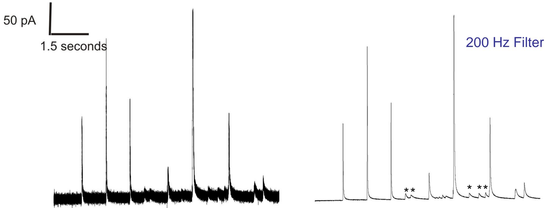
Filter cut-off frequencies must be chosen carefully and vary by cell type.
