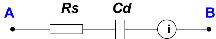
Circuit Model with  $R_s$  representing solution resistance and  $C_d$  for double layer capacitance at the electrode surface
