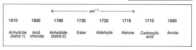
it looks as though the expected frequency of an ester, 1735 cm<sup>-1</sup>, is closest to our observed peak frequency. This is great, because it explains the two oxygen atoms in the molecular formula.
