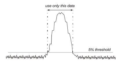
In addition, if your GPC graph shows multiple independent peaks in different molecular-weight regions, you might want to calculate  $\overline{M_n}$ ,  $\overline{M_w}$  and PDI for each peak independently.
