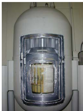
Interior of a 4.73 T magnet (on display in NMR Facility, Smith Hall)
