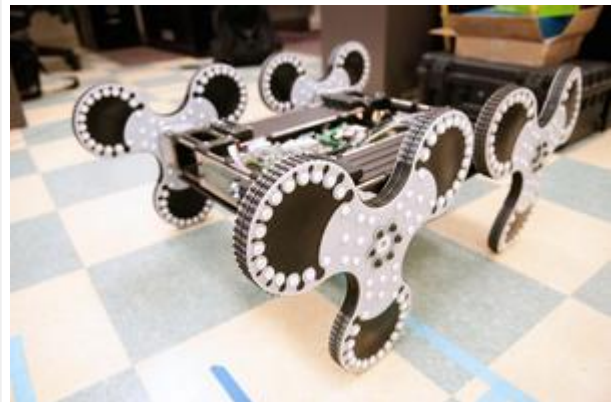
The "loper" crawls across the floor of the Center for Distributed Robotics lab Friday in Wilson Library. The loper was designed to travel over large obstacles and has the ability to ascend and descend stairs with ease. SATCHELL MISCHÉ-RICHTER
