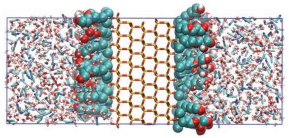
The figure shows the simulation system, which uses a slit pore model. This system consists of a silica support with a diol stationary phase grafted to the surface as well as freely floating water and acetonitrile molecules, which act as the mobile phase. The colors yellow, red, teal, white, and blue correspond to silicon, oxygen, carbon, hydrogen, and nitrogen molecules respectively.
